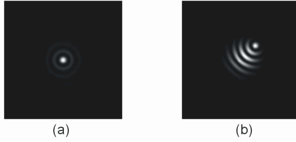
Fig. 3. The intensity spot of the B-G beam at (a) the on-axis and (b) the off-axis positions.
