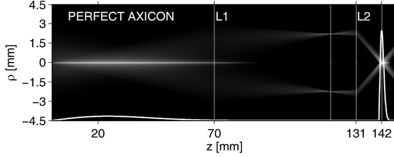
Fig. 3. A free-space propagation method was used to calculate the spatial optical intensity distribution of the field behind the perfect axicon illuminated by a Gaussian beam (beam waist  $w_0 = 2140 \mu\text{m}$ ) at the wavelength  $\lambda = 1064 \text{ nm}$ . The telescope is formed from lenses  $L_1$  and  $L_2$  of focal lengths  $f_1 = 50 \text{ mm}$  and  $f_2 = 11 \text{ mm}$ , respectively. The white curves show the numerically calculated axial intensity profiles.
