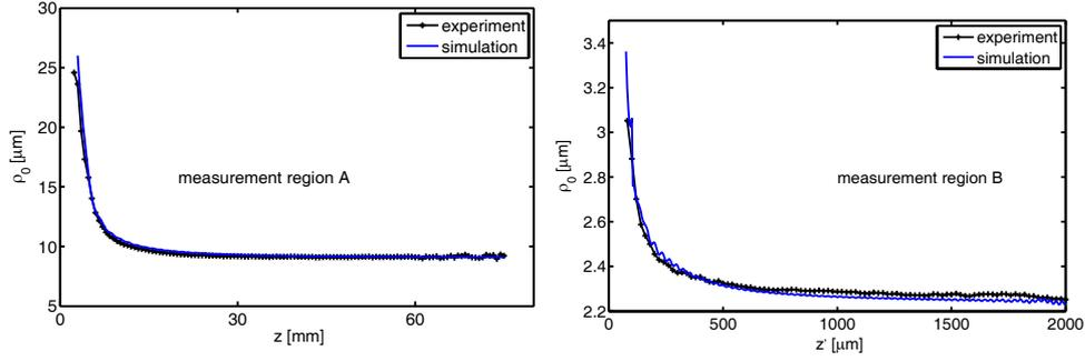
Fig. 8. Comparison of measured and calculated radius  $\rho_0$  of the high intensity QBB core generated by the round-tip axicon measured directly behind the axicon (left) and behind the demagnifying telescope (right).
