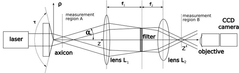
Fig. 6. Experimental set-up. Laser: IPG, YLM-10-1064-LP, wavelength 1064 nm, maximal power 10 W, beam-waist of incident Gaussian beam  $w_0 = 2140 \mu\text{m}$ ; axicon: EKSPLA 130-0270, apex angle  $\tau = 170^\circ$ ; lenses  $L_1, L_2$ : focal lengths  $f_1 = 50 \text{ mm}$  and  $f_2 = 11 \text{ mm}$ ; objective: Mitutoyo M Plan Apo SL 80X; CCD camera: IDT X Stream VISION XS-3.
