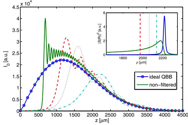
Fig. 10. Calculated axial intensity profile for perfect axicon (open circle with full line), and round-tip axicon with  $a = 33.7 \mu\text{m}$ . Different radii  $R_f$  of the spatial filter placed in the Fourier plane were considered:  $0 \mu\text{m}$  (full),  $1973 \mu\text{m}$  (dashed),  $2064 \mu\text{m}$  (dotted), and  $2138 \mu\text{m}$  (dot-dashed) (see the inset for corresponding spatial frequency spectrum cut-off).
