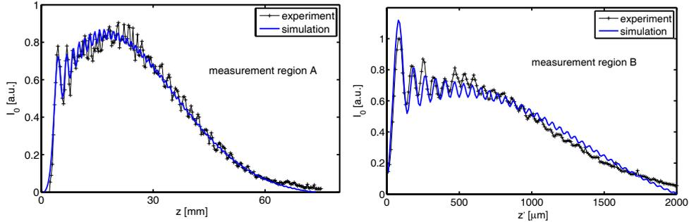
Fig. 7. Comparison of measured and calculated axial intensity profile  $I_0$  of the QBB generated by the round-tip axicon measured directly behind the axicon (left - measurement region A in Fig. 6) and behind the demagnifying telescope (right - measurement region B).
