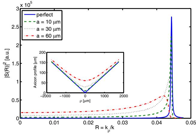
Fig. 4. The spatial-frequency spectrum  $|S(R)|^2$  of the field behind the perfect axicon and axicon with round tip calculated for the Gaussian beam waist  $w_0 = 2140 \mu\text{m}$ , the wavelength  $\lambda_{\text{vac}} = 1064 \text{ nm}$  and the apex angle of the axicon  $\tau = 170^\circ$ , and axicon refractive index  $n = 1.50669$ . The hyperbolic shape of the axicon tip (see the inset) creates low frequency components in the spatial-frequency spectrum.
