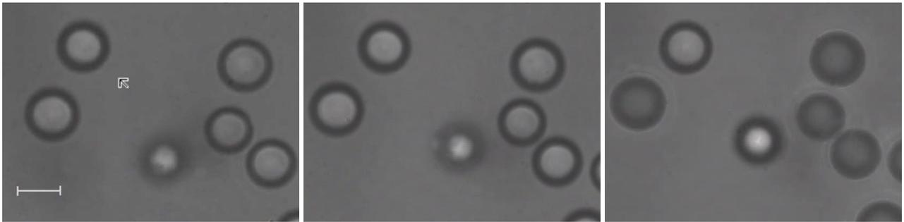
**Figure 5.** Arrow signed polymer microsphere with diameter  $5 \mu\text{m}$  (4k-5 Duke Scientific) is trapped by COP in water solution. Particle is trapped by COP among particles of the same size and it moves towards to cover slip by vertical movement of the microscope objective. Sharpness of surrounding particles is changing. Power in the focal point is 55 mW. Vector on the first picture has length  $5 \mu\text{m}$ .
