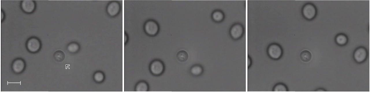
**Figure 10.** Manipulation with yeasts *Saccharomyces cerevisiae* (arrow signed), trapping power 30 mW. Yeast is trapped by COP and the sample moves transversally. Yeasts laying on microscope slide are moving to the bottom of the image, trapped yeast has same position. Vector on the first picture has length 5  $\mu\text{m}$ .
