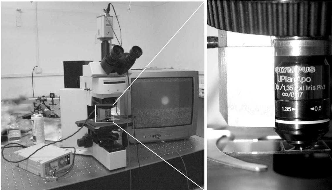
**Figure 8.** COP mounted on the upright microscope Olympus BX-50. View of the apparatus and current controller (left) and detailed view of the COP (right).
