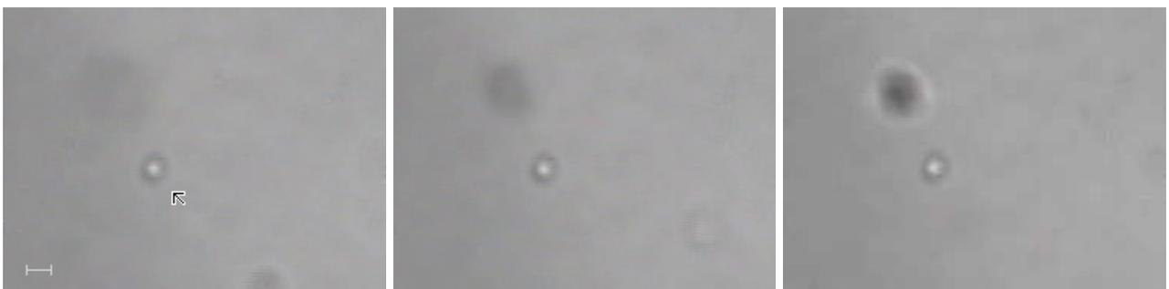
**Figure 7.** Arrow signed polymer microsphere with diameter  $520 \text{ nm}$  (3k-500 Duke Scientific) in water solution is trapped by COP. The position of the optical trap is changed by vertical movement of the microscope objective and image on CCD camera focuses. Power in the focal point is 55 mW. Vector on the first picture has length  $1 \mu\text{m}$ .
