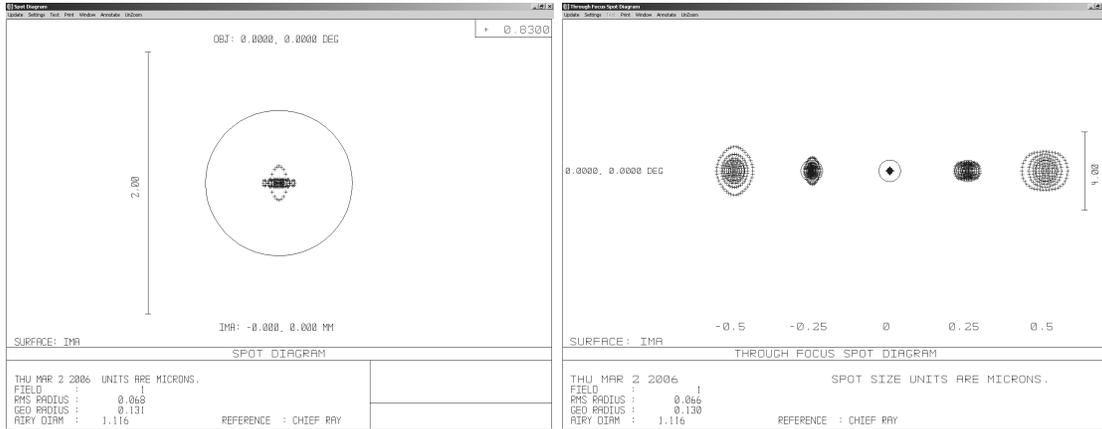
Figure 1. Spot diagram (left), through focus spot diagram (right) from Zemax optical program.
