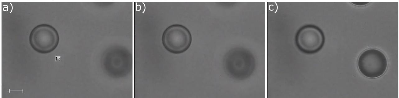
**Figure 4.** Arrow signed polymer microsphere with diameter  $10 \mu\text{m}$  (4k-10 Duke Scientific) is trapped by COP in water solution. Object in the right part of images a) and b) laying on the microscope slide is blurred. Position of the optical trap is changed by vertical movement of the microscope objective and the image of the right particle is focused c). Trapped particle stays focused. Power in the focal point is 55 mW. Vector on the first picture has length  $5 \mu\text{m}$ .
