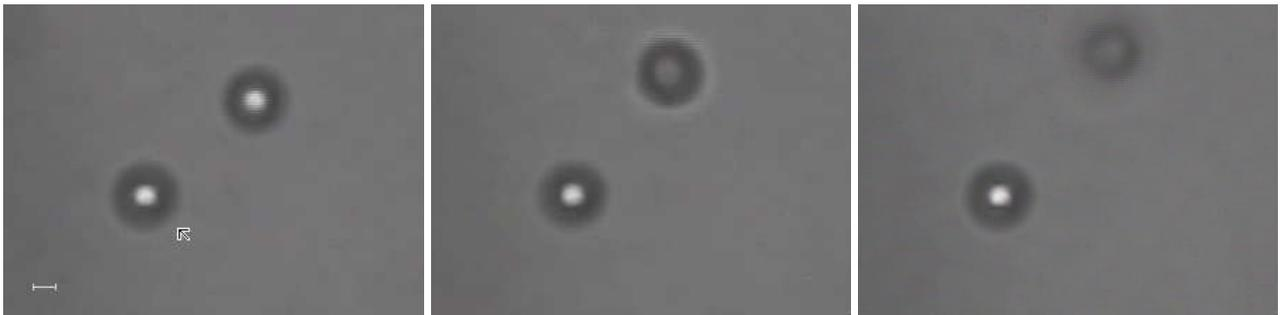
**Figure 6.** Arrow signed polymer microsphere with diameter  $2 \mu\text{m}$  (4k-2 Duke Scientific) in water solution is trapped by COP. Object in right part of left image laying on the microscope slide is focused. The position of the optical trap is changed by vertical movement of the microscope objective and image of the right particle blurs. Trapped particle stays focused. Power in the focal point is 55 mW. Vector on the first picture has length  $1 \mu\text{m}$ .
