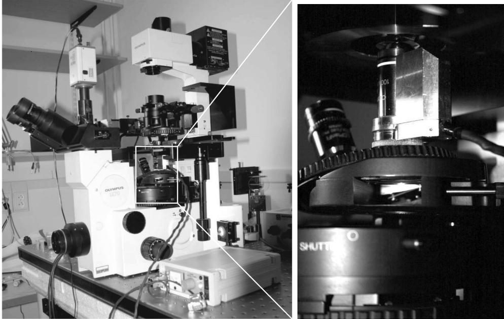
**Figure 3.** COP mounted on inverted microscope Olympus IX-70. View of the apparatus (left) and detailed view of the COP (right).
