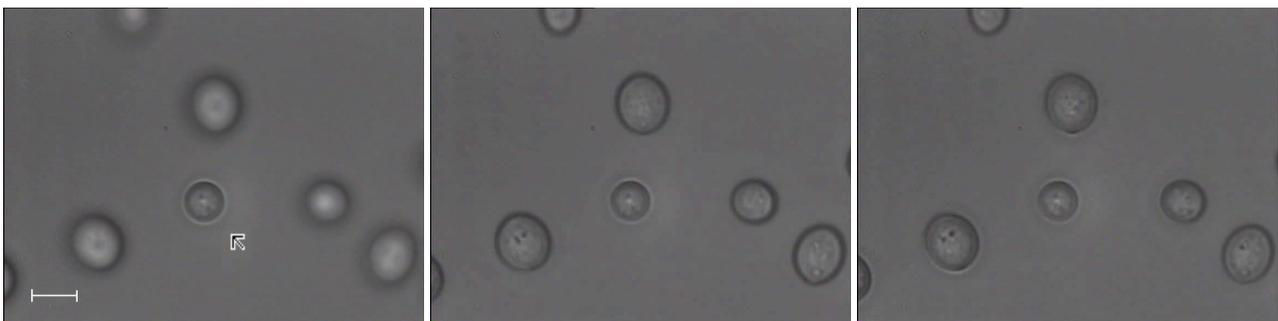
**Figure 9.** Manipulation with yeasts *Saccharomyces cerevisiae* (arrow signed), trapping power 30 mW. Yeast freely levitating in water solution is trapped by COP and the sample moves longitudinally. The image of the yeast is still focused, while the yeasts laying on microscope slide sharpen. Vector on the first picture has length 5  $\mu\text{m}$ .
